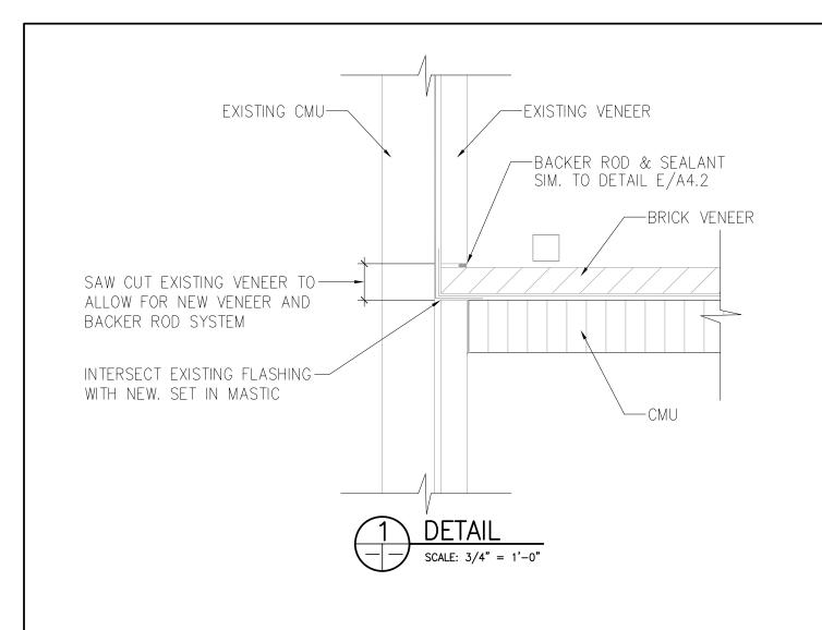
ADDENDUM #3 ATTACHMENT 'A' WALL FLASHING DETAIL
